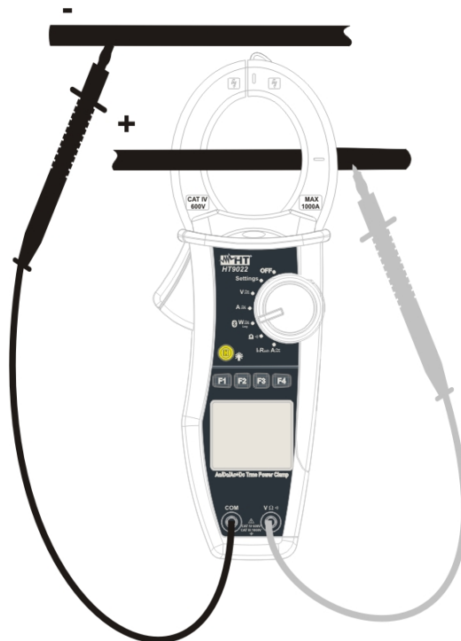
Fig. 11: DC power measurement
