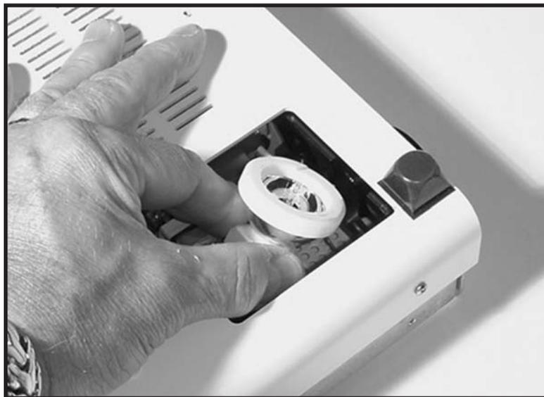
Use the above procedure in reverse order to insert the new bulb. When installing the new bulb, be sure to align the pin on the outer rim of the lamp with the groove in the mating hardware inside the unit.
