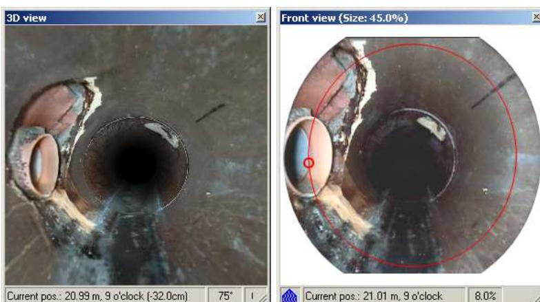
Figure 11: 2 front views at the same position of a DigiSewer scan: 3D view window (left) and the frontview window (right).
