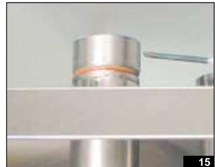
Make certain that the upper oven vent remains closed (fig. 15). Ensure that there are no leaks onto the oven conduits and condensation/steam generation system.
