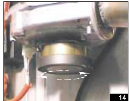
Turning it clockwise increases the frequency and hence the **speed of the fan during the ignition phase.**
