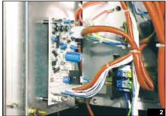
Setting a cooking temperature higher than the temperature in the oven causes the closure of the voltage-free clean contact 4-5 (X3), which acts as an ON-OFF control.
