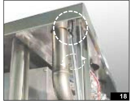
The oven cover is now free from all obstructions. Use a spacer to keep the cover raised above the oven, as this will later facilitate removal of the boiler (fig. 19-20).
