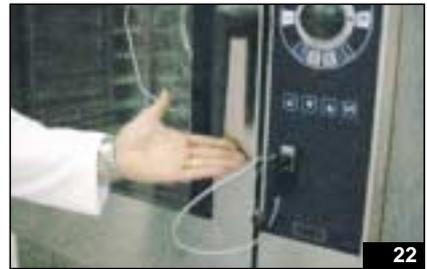
When cooking is complete, remove the core probe from the food and unplug the male connector from the female socket on the control panel by pressing the release mechanism at the top (fig. 23).
