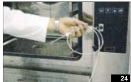
Warning: do not run the cable into the oven in the area around the door closure mechanism, as this could damage it (fig. 26).
