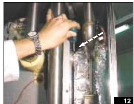
Using the screwdriver, unscrew the clip securing the top of the steam input sleeve (between the oven and the boiler), until the clip turns freely (fig. 12-13).
