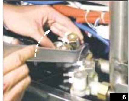
**4th phase:** Remove the solenoid valve water intake filter and clean it (fig. 7-9).
