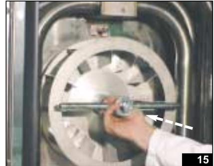
**6th phase:** Insert the motor fan puller, and using the 24 mm wrench to turn the central pin of the puller, remove the fan.
