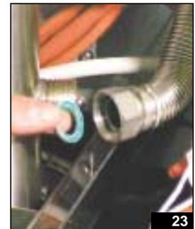
Disconnect the boiler water filling conduit, using a 10 mm wrench, and pulling the connecting joint towards the outside of the boiler (fig. 24-25). For further details, see section 13.1.
