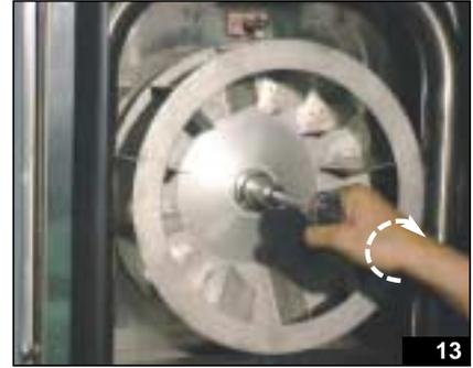
**5th phase:** Using the 19 mm T-wrench, unscrew the motor spindle screw by turning it **clockwise** (NB the screw has a left-hand thread) and remove it (fig. 13-14). Avoid forcing the fan blades as this could affect their balance.
