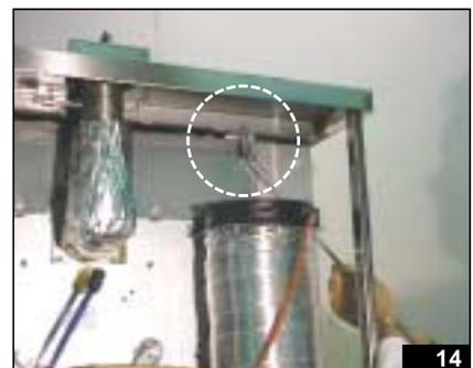
Unscrew the descaler inlet plug located in the right-hand corner of the oven ceiling, and remove the gasket (fig. 15-16).
