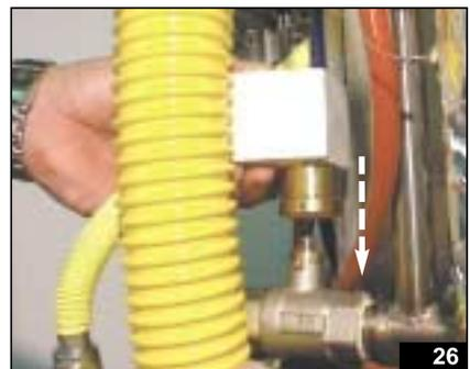
Carry out a test in steam mode in order to check that the water/gas/steam injection circuit is properly sealed.
