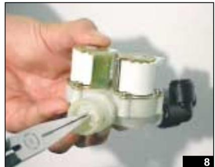
This done, check that no water leaks from the valve casing and that the plastic water conduits are inserted as far as they will go, into the black plastic sealing joint.
