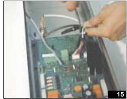
Now that the control panel is free from any obstructions, lay it on a flat surface to facilitate replacement of the electronic card.
