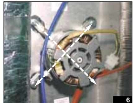
**5th phase:** After centering the motor, fasten the 4 screws in diagonally opposite sequence, and check manually that the motor spindle turns freely (fig. 5).
