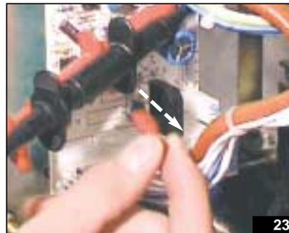
At this point, by selecting **low fan speed** from the control panel (fig. 25), the fan switches on at minimum speed, which must be adjusted by means of the trimmer (Min Hz) to 112 Hz (MG 101 - G20) in accordance with the table (fig.26).
