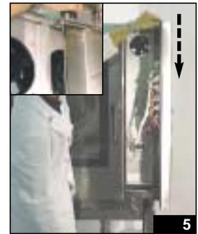
This leaves the control panel open like a book and enables you to reset the oven safety thermostat F2 and the boiler safety thermostat F3 (fig. 6).
