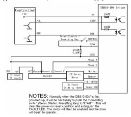
Figure 4: Typical connection (Using external +5V to supply the encoder)
