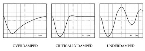
Figure 6: Response to an impulse load
