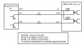
Figure 2: Control signal connection
