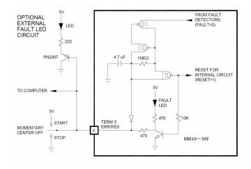
Figure 7: Error clear and Reset circuit of the DB810-50V
