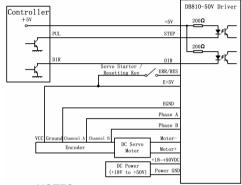
NOTES: Normally when the DB810-50V is first powered up, it will be necessary to push the momentary switch (Servo Starter / Resetting Key) to START. This will clear the power-on reset condition and extinguish the FAULT LED. The motor will then be enabled and the drive will havin to operate
