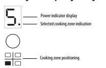
Once the hob is switched on and the pan is positioned on the chosen cooking zone, select the zone using the corresponding button: the display shows level 5.
