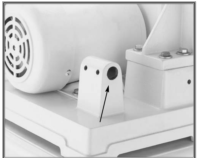
Figure 25. Working table mounting hole when vertical sanding.
