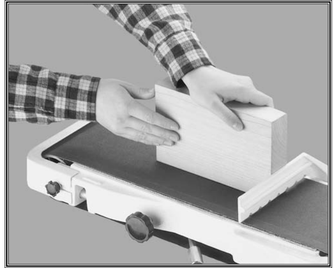
Figure 32. Sanding with back stop.
