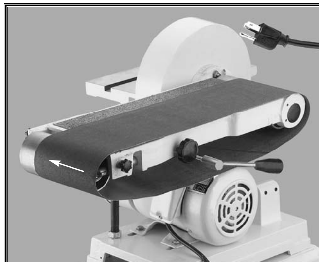
Figure 18. Installing the sanding belt.
