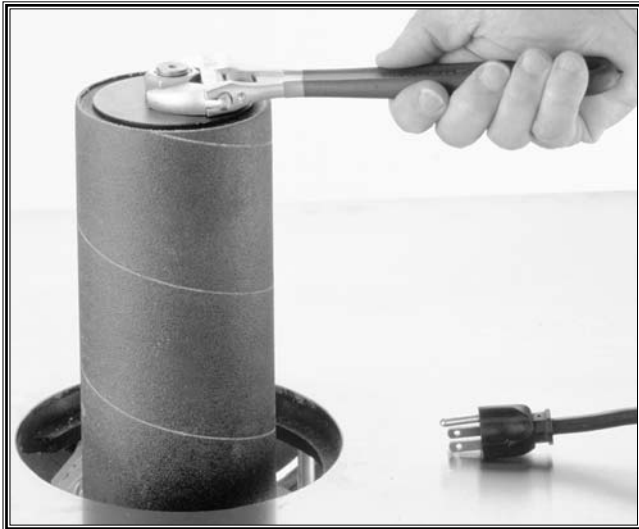
Figure 11. To remove the sanding sleeve from the spindle, loosen the hex nut on the top of the spindle.
