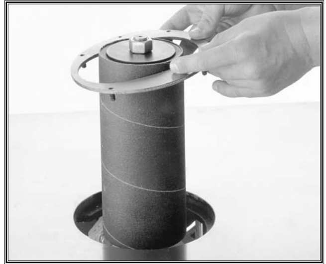
Figure 13. The table insert should clear the spindle by at least \frac{1}{8} " on all sides. Pins on the underside of the insert ensure correct positioning in the table.
