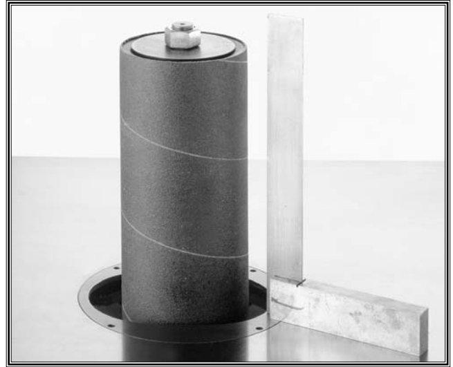
Figure 17. Use a machinist square to adjust the table square to the spindle.
