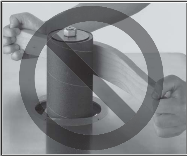
Figure A. Never sand a workpiece while holding it off the table surface.
