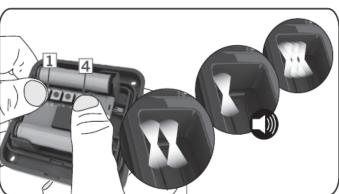
PRESS THE CHANNEL IN WHICH THE FINGERPRINT WILL BE PROGRAMMED
