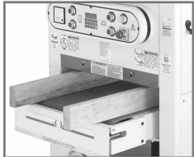
Figure 18. Gauge boards placed under pressure rollers as a gauge.
