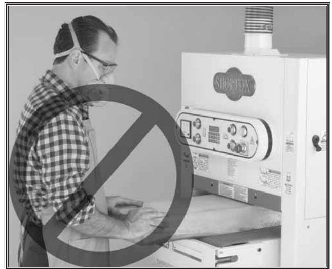
Figure 3. DO NOT stand behind workpiece!
