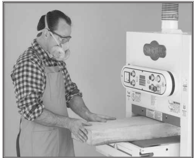
Figure 29. Operator feeding workpiece in correct body position and out of the way of potential kickback.
