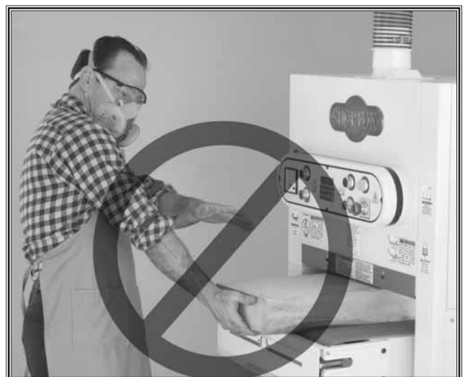
Figure 5. DO NOT allow hand to get pinched in belt!
