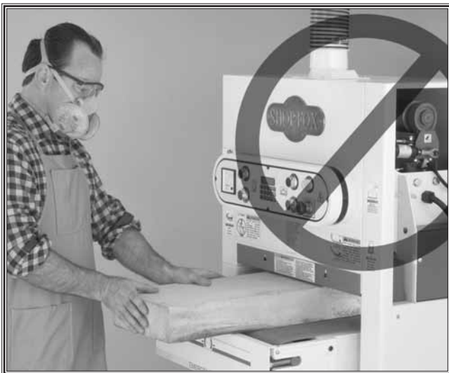
Figure 4. DO NOT operate with side door open!
