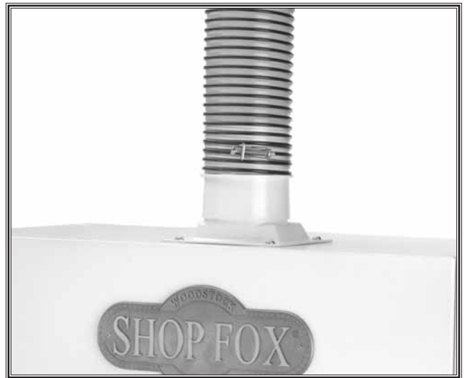
Figure 11. Dust collection hose attached to dust port.
