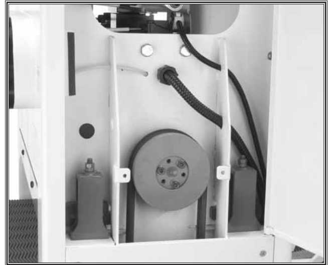
Figure 37. Upper pulley exposed.
