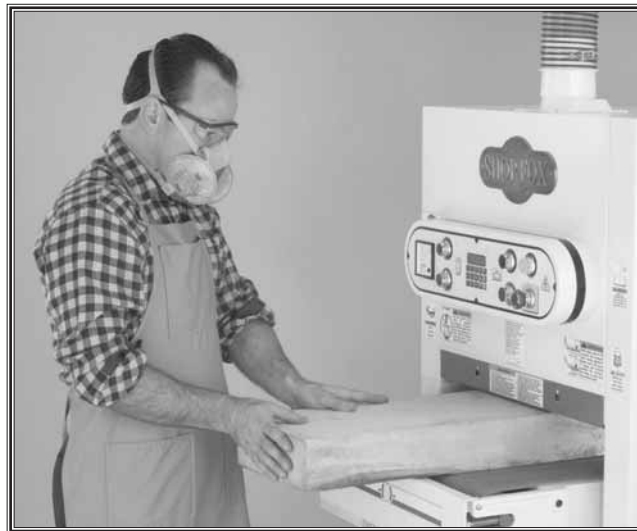
Figure 1. Correct body and hand positioning.
