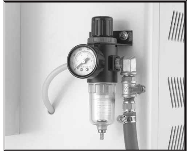
Figure 7. Air hose attached to regulator.
