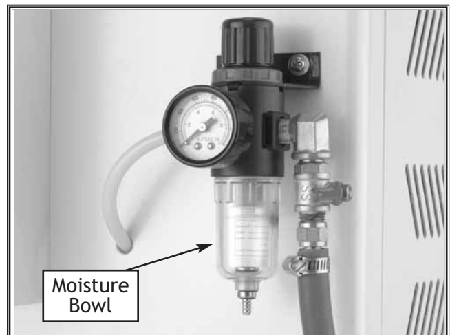
Figure 34. Drain the moisture bowl often.
