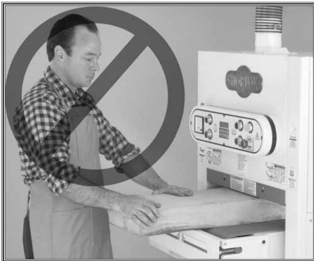
Figure 2. DO NOT operate without safety glasses/respirator!
