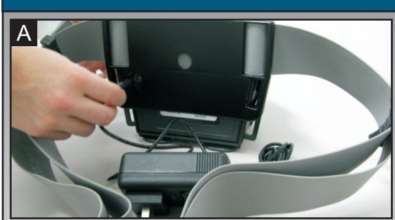
**A.** Plug battery charger into socket at back of the battery pack and connect to an electrical outlet. Charge battery pack for approximately five hours before use. The battery charger LED will flash green when charging is complete.
