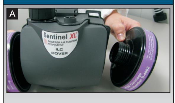
A. After Decon, turn filters counterclockwise. Unscrew filters and discard. Before installing new filter check gasket for any damage.
