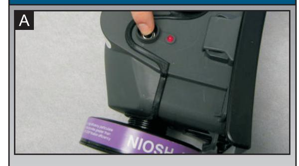
**A.** Depress switch on top of blower. A short beep should sound and light the red LED continuously.
