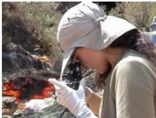
Nikon model H field microscope being used by Dr. Amaral-Zettler to observe protists at the Origin site. © Erik Zettler and Linda Amaral Zettler
