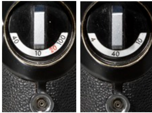
The 100x lens can be replaced by a DLL 20x shown added in red. The selector pulls out and rotates to show the other, standard 4-40-10 option.
