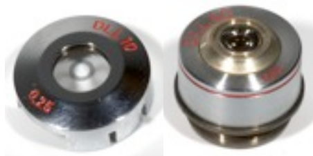
The 40x lens has its stop built-in while the 10x lens actually has a slip-on one that can be removed.
