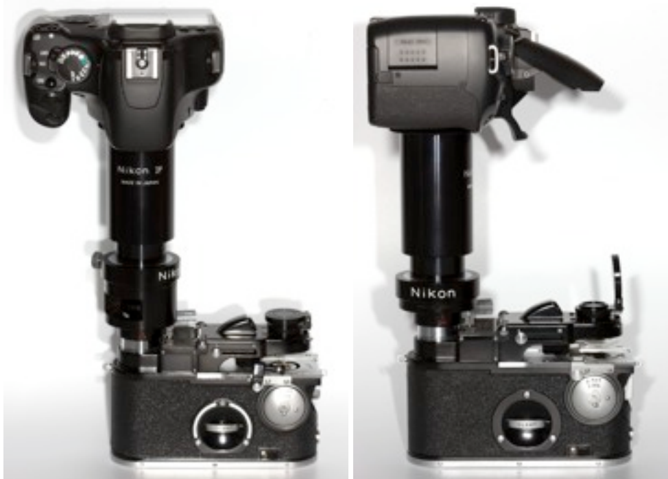
The 1960s F camera adapter still works fine today and a camera's built in flash can be used for illumination without effort.
