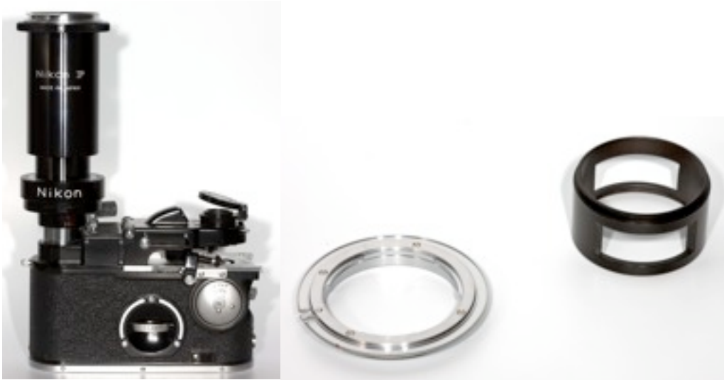
The Nikon F camera adapter - A Nikon F to Canon EOS adapter ring - The filter holder of the Nikon F camera adapter. Glass filters are just dropped in. Three different colours were supplied.
