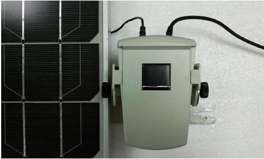
Connect the Solar panel (front side) with Irradiance meter
