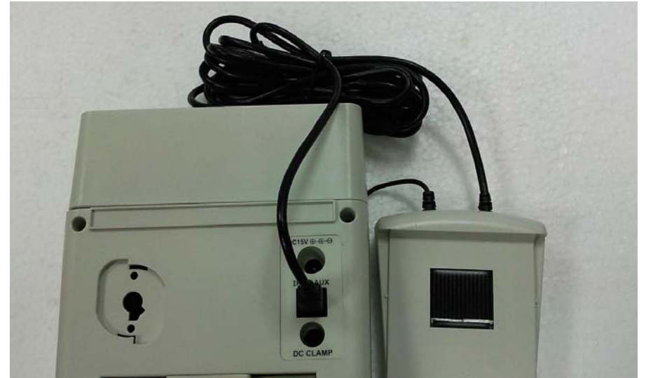
Connect Analyzer with Irradiance meter
