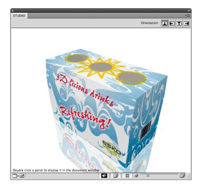
If the placed ARD file does not contain folding angles, the plug-in cannot know how the box has to be folded. In that case 90-degree foldings are assumed on all folding lines. If the resulting shape is not the intended one, the proper folding angles need to be added to the ARD file, for example using ArtiosCAD or Studio Toolkit for Boxes.
