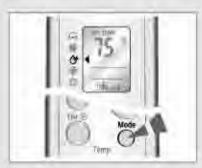
2 Press the button on the remote control until of is displayed.
