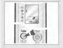
You can select the Turbo Function if you want to cool or heat your room in the fastest way. After the 30 - minute operation with the maximum setting, it returns to the previous setting.
