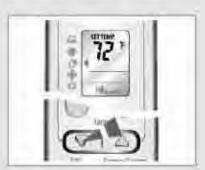
3 Press the V | A button to adjust the temperature until the required temperature is displayed. You can set the temperature between 61°F(16°C) and 86°F(30°C).
