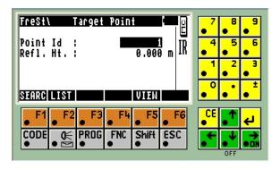
Once these two points have been shot use the **F6** button to access the **CALC** function. This will do the math for the total station to figure out where it is set up upon. The total station will know spatially where it is located so that it can measure and calculate more unknown points within the survey area.
