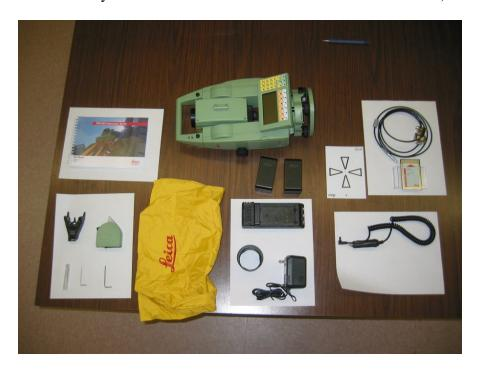
The contents in our TCR1105 case are displayed in the photo above, clockwise starting with top left corner are; basic user manual, TCR1105 total station unit and 2 batteries, target plate, computer serial cable, flash card, car charger, AC power cord, battery charger, lens cover, weather cover, height meter (measuring tape and customized plastic hook), and various allen hex keys.
