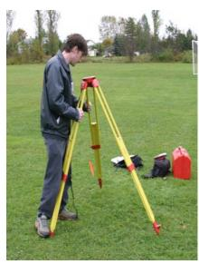
Next place the tripod approximately centered over top of the point on the ground and as level (it will be fine tuned later but it makes it easier if you start off close to level) as possible with the legs evenly spread out wide enough to provide adequate stability.
