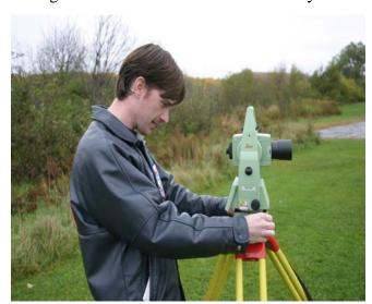
combination allow the device to calculate the location of the instrument with GPS satellites and then use that spatial information along with the total station tools to measure and calculate spatially referenced values for the other unknown points.
