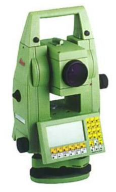
m, a distance error would vary from 3 mm to 15 mm over this range of accuracies. The total distance that the EDM can measure depends on a number of variables, including atmospheric conditions, quality of the EDM, and the number of prism reflectors used as targets over top of the destination points.
