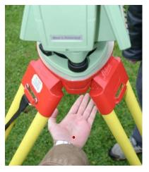
The electronic level works similar to the bubble level that is found on a typical survey tribrach. You want to have the small levelling circle contained within the cross hairs of the target circle on the display screen.
