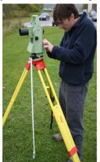
Attach the **spacing bracket** to top of one of the foot screws as illustrated right. This will hold the end of the height meter (tape measure).
