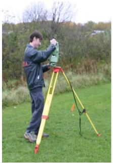
Plant one of the three legs firmly into the ground with your foot using the peg on the end of the leg for assistance.
