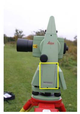
**Tip:** None of Leica's survey equipment used ever needs to be forced to fit into any of the slots. If a piece of equipment does not seem to want to "fit" properly it may not be oriented correctly for insertion. So it is better to take your time and Check again!
