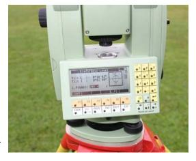
With the laser plummet on, grasp the other two legs of the tripod and use them to orient the laser over point on the ground plummet.
