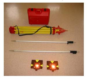
Other equipment used in the operation of the unit are displayed in the photo on the left and include a survey grade tripod, reflective survey prisms and aluminum poles with height measurement labelled and built in level bubbles to mount the prisms onto. The reflective survey prisms can also be used with survey grade tripods (shown below) when mounted on tribrachs.
