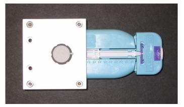
For pullout force measurements the capstan is replaced by the toggle clamp assembly.
