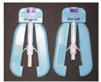
This modification permits the tool to be held in the holder by a pin. The photograph below shows the tool inserted in the holder, as shown below. The knob in the middle of the holder attaches to the pin. The pin has a flat on it which seats firmly against the frame of the stripping tool.
