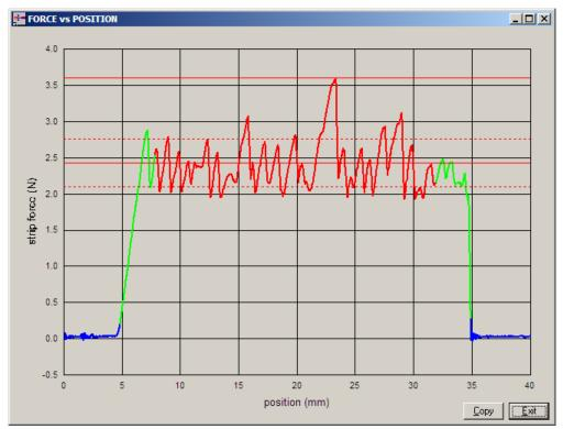
The graph window provides a detailed view force/position data captured during the experiment. <u>Only the</u> <u>red part of the trace</u> is used to calculate the maximum, mean and standard deviation of the strip force.
