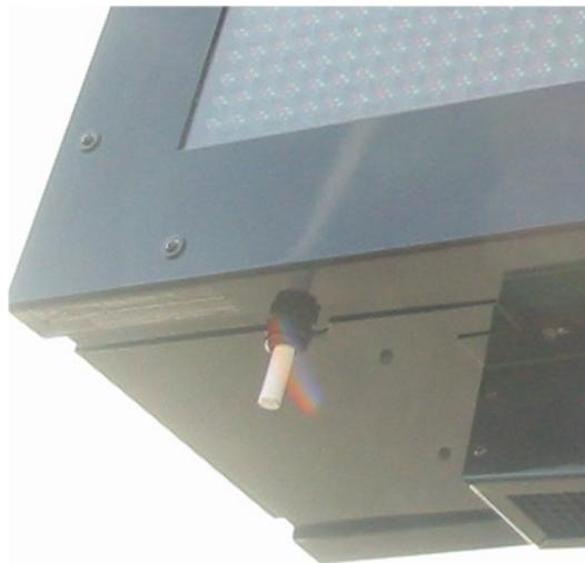
**Figure #14 - The Temp Probe is Located at the Bottom Left of ID# 1**
