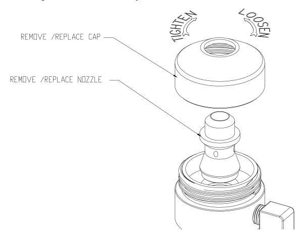
Remove the spray gun cap, remove the nozzle, and replace with one of a larger size.
