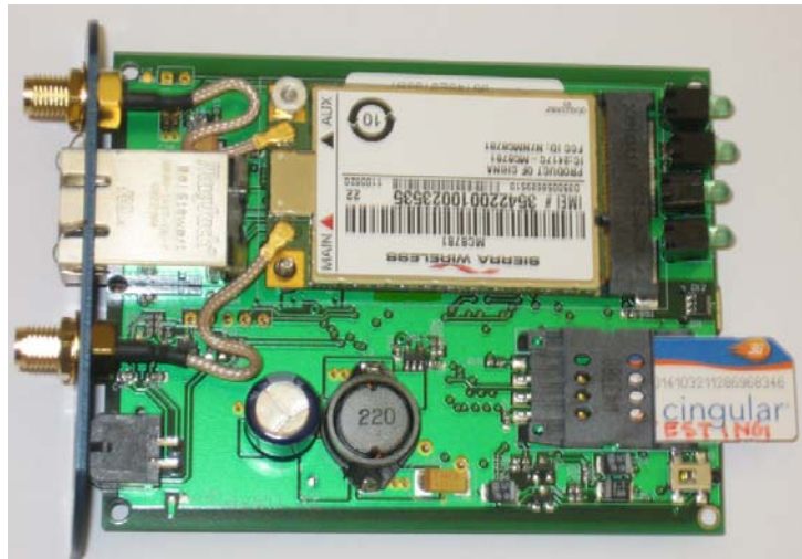
Figure 3-3: Insert SIM in to the modem
