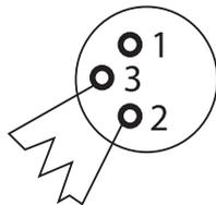
Termination reduces signal transmission problems and interference. it is always advisable to connect a DMX terminal, (resistance 120 Ohm 1/4 W) between pin 2 (DMX-) and pin 3 (DMX+) of the last fixture.
