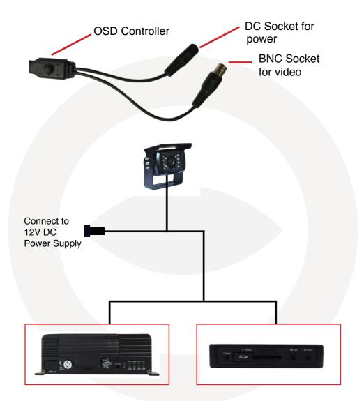
Connect to any camera input device that supports BNC (as shown above)\*.
