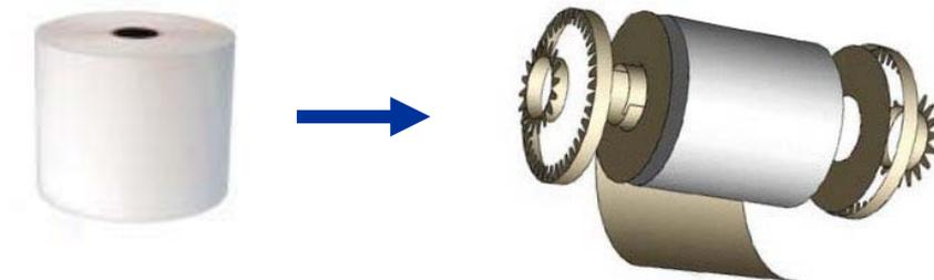
Paper roll will rotate and come out once the “FEED” button is pressed.
