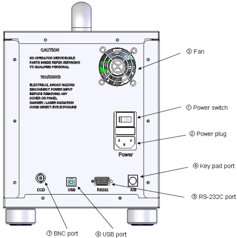
Figure 4. The rear side of the main device
