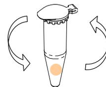
4. Load 20  $\mu$ l (for SCC kit CRS-K01, 2 channel chip) or 12  $\mu$ l (for SCC kit CRS-K02, 4 channel chip) of the cell sample onto the Chip. Ensure that no bubbles enter the channel.
