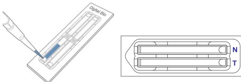
**Insert the chip into the chip holder and push the run button.**
