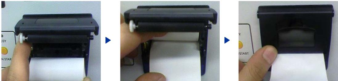
Figure 5. The method of paper roll refill
