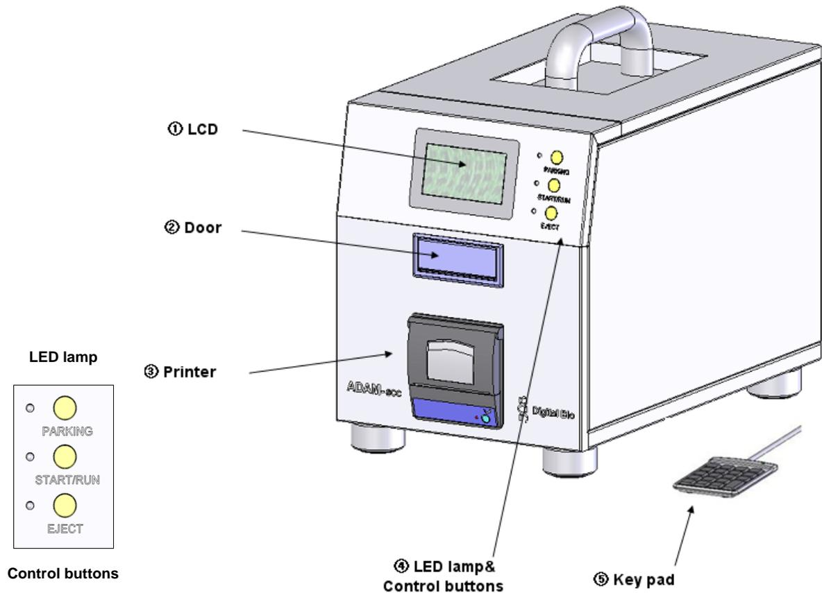
Figure 2. The front side of the main device
