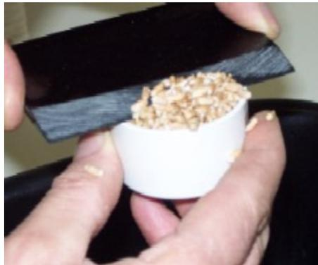
Figure 5: Levelling the Cup
