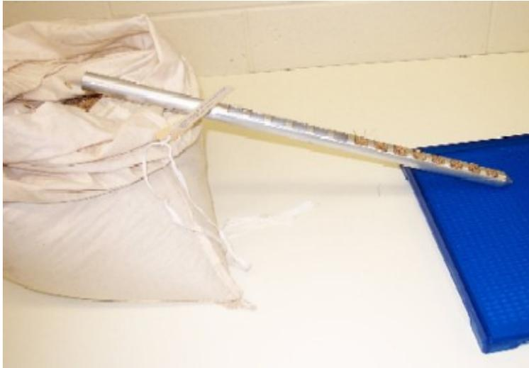
Figure A-2: Tube Ready to Invert and Fill Sample Cup
