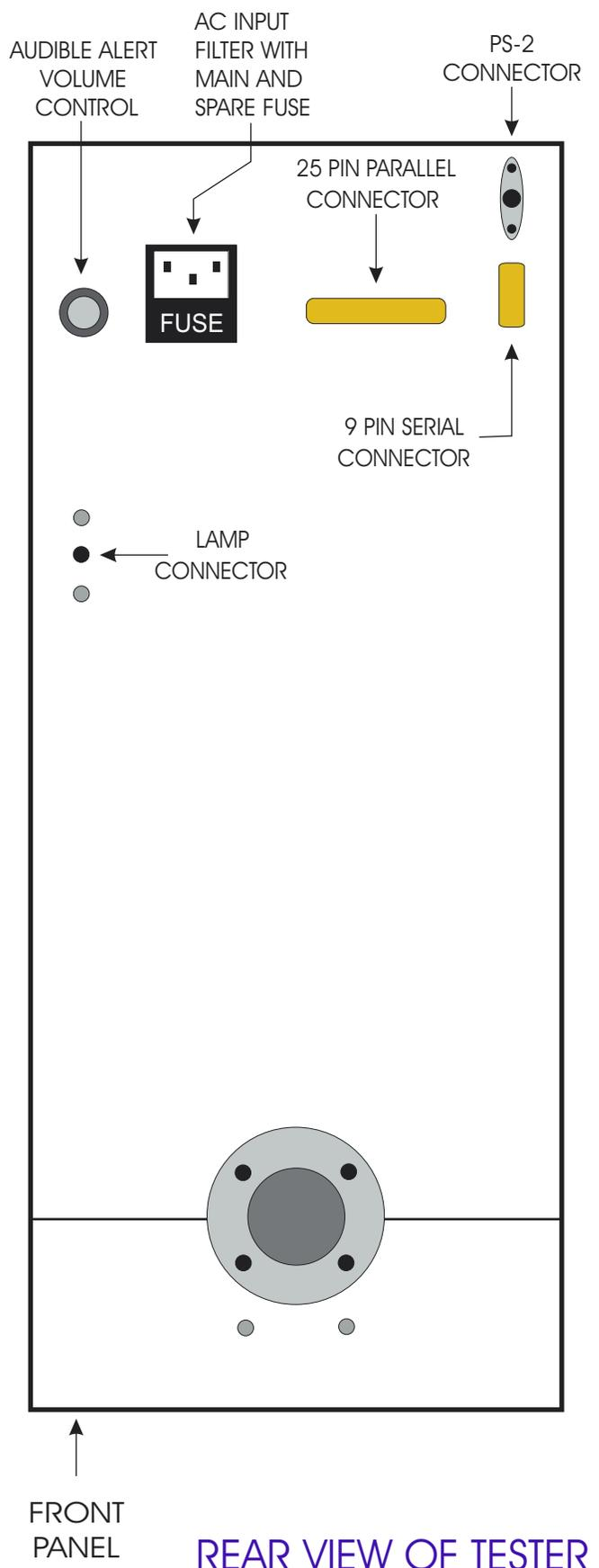
REAR VIEW OF TESTER AND BOTTOM OF HEAD
