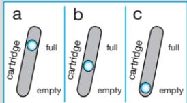
The display for cleaning fluid (6) will show how much cleaning fluid is in the cartridge:
