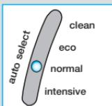
If the system has selected one of the three cleaning programs, it will not start until you push down the «start cleaning» button (2). This locks the shaver into the station and starts the cleaning process.
