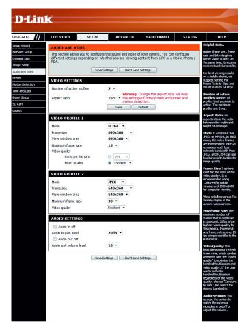
This limits the maximum frame rate, which can be Video Quality: combined with the "Fixed quality" option to optimize the bandwidth utilization and video quality. If fixed bandwidth utilization is desired regardless of the video quality, choose "Constant bit rate" and select the desired bandwidth.
