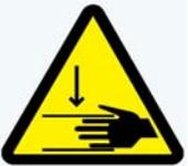
**Never** hold to the frame of covers or brackets while closing the UC. **Always** use special handle. Holding your hand in improper place can result a sever injury. **Crush Hazard**
