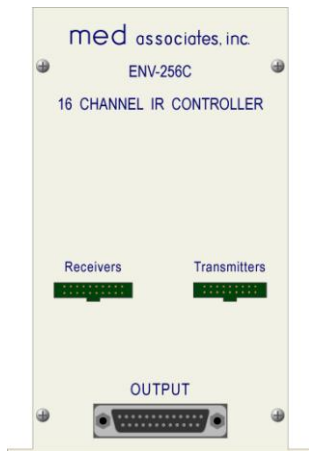
Figure 2-2 - ENV-256C 16 Channel IR Controller
