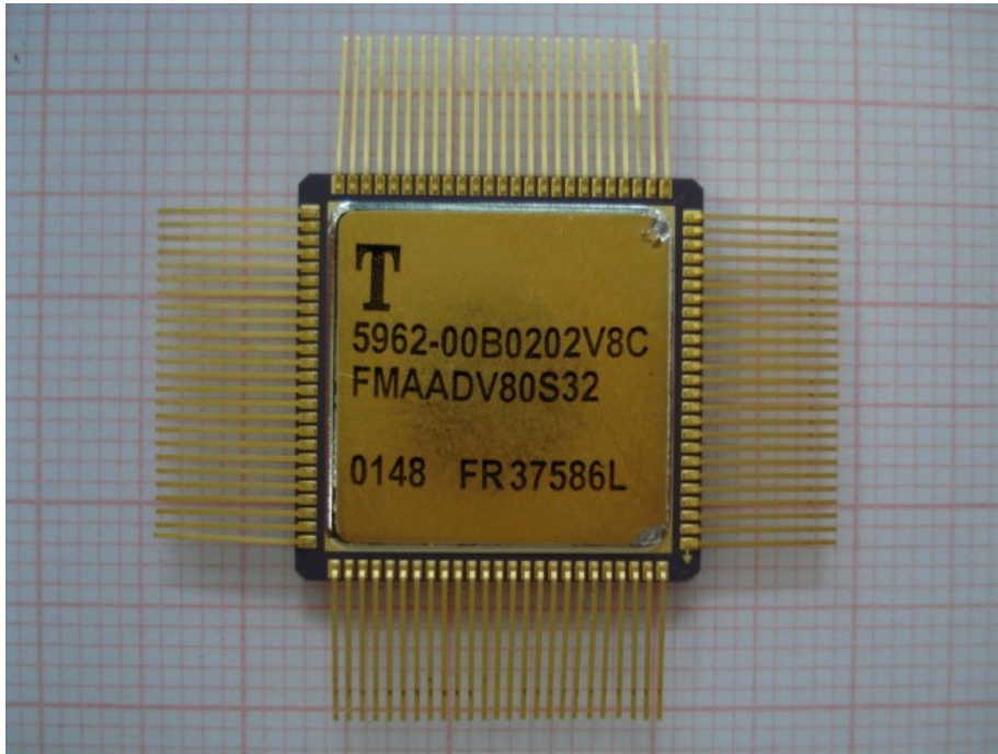
Figure 10.1: 80S32 DUT lidded and top marking
