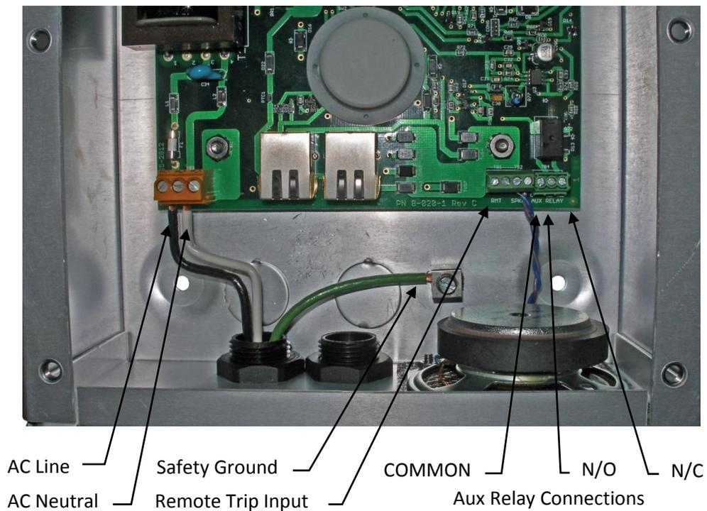
13. Install the shunt on JP1. (Refer to step 3.) Replace the case and test the system. Apply caulk sealant to the case to wall interface along the top edge of the case especially if the wall is not smooth such as lap siding or corrugated metal.
