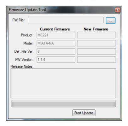
The connected devices details are shown on the left boxes, including its product code, type and definition file version, as well as the current firmware version on the device.
