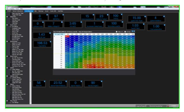
On the default 'Grid View' (above), the current input data points are shown by the cross hair intersection formed by the yellow lines - and note that it also considers real-time interpolation to correctly show how far the engine or connected system is from the 'centre' of the current cell.
