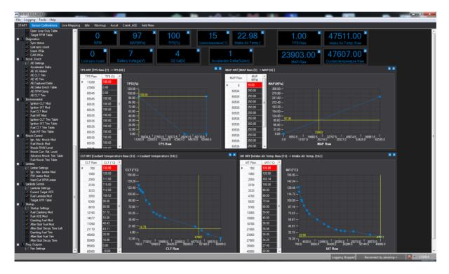
Yellow lines and text on the view show the current 'real' results that are being used in the ECU (when online).
