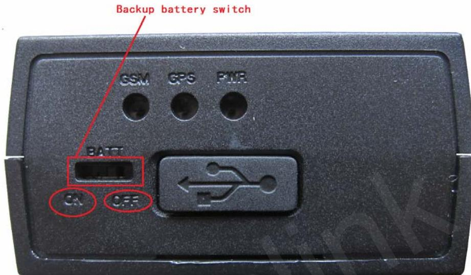
**Figure 7. Switch and ON/OFF position**
