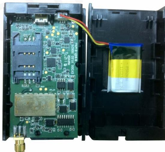
Figure 6. Backup Battery Installation
