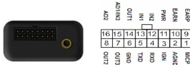
Figure 2. The 16 PIN connector on the GV300
