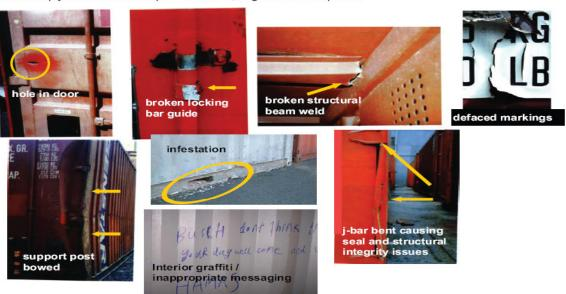
Cargo container doors should seal completely and securely when shut. The container should be light-tight, which will also prevent entry of any external elements into the container while in transit. To ensure a satisfactory light-tight seal, you can conduct a light test by observing the seal performance from inside a closed container. In addition, all door locking hardware (hasps, hinges, handles, bars, bolts, etc.) must be tested and be in good working order (see below diagram).
