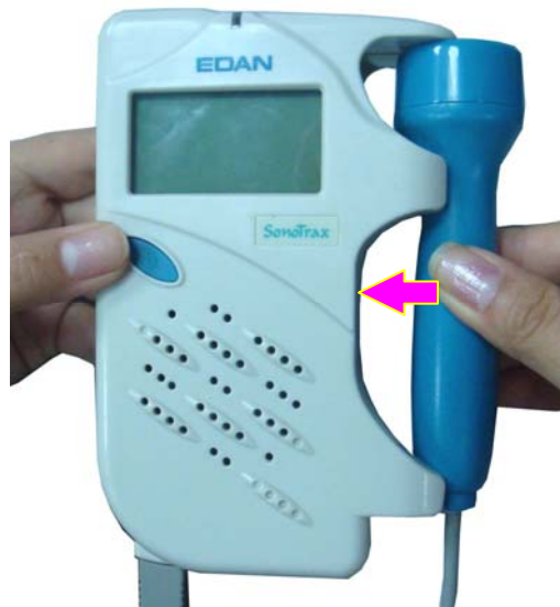
Figure 3-5 Placing the probe
