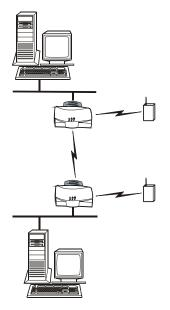
• as a repeater to extend coverage area without additional network cabling
