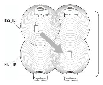
APs with the same Net\_ID (ESS) define a coverage area. The MU searches for APs with a matching Net\_ID (ESS) and synchronizes with an AP to establish communications. This allows MUs within the coverage area to move about or *roam*. As the MU roams from cell to cell, it switches APs. The switch occurs when the MU analyzes the reception quality at a location and decides the AP to communicate with based on the best signal strength and lowest MU load distribution.
