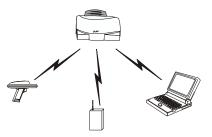
• A single AP can bridge the Ethernet and radio networks.
