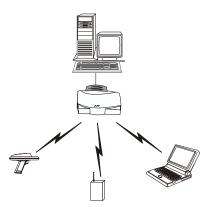
• Multiple APs can coexist as separate, individual networks at the same site without interference using different Net\_IDs.
