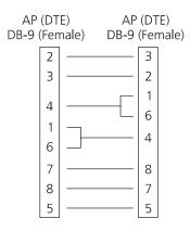
Connecting two APs with modem devices requires straight-through cables between the APs and modems. Using modems requires a telephone line for as long as the link remains active.
