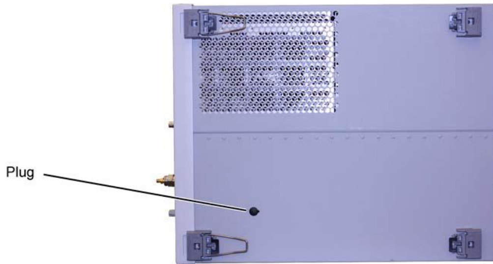
Figure 3. Removing the Timebase Adjustment Access Plug
