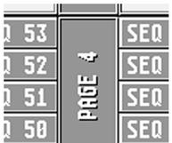
After pressing the LIST button once, the TFT display will show a listing of the Sequences assigned to the Buttons, and in the middle a PAGE Button with the currently called-up EXECUTOR Page.
