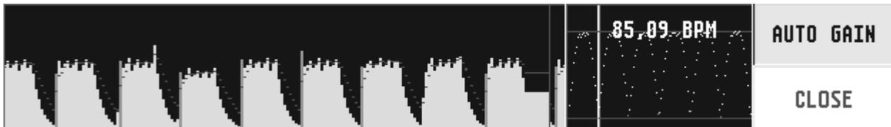
The right small dot will indicate the state of compression of the audio signal. The sound signal is visualized in the lower left part of the display. The analysis of the sound signal will be indicated in the smaller right part of the window, including indication of the recognised BPM (Beats per minute). By moving the BPM slider, the beats per minute can be adjusted.
