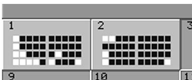
The buttons are indicated by symbols in the respective PAGE buttons. If there is a green square, a Sequence, a Group or a Special Master is allocated to this Executor Button. If this square is yellow, the Sequence or Chaser is active.
