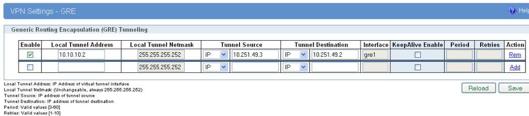
Figure 54 - GRE configuration page for GWR Router 2
