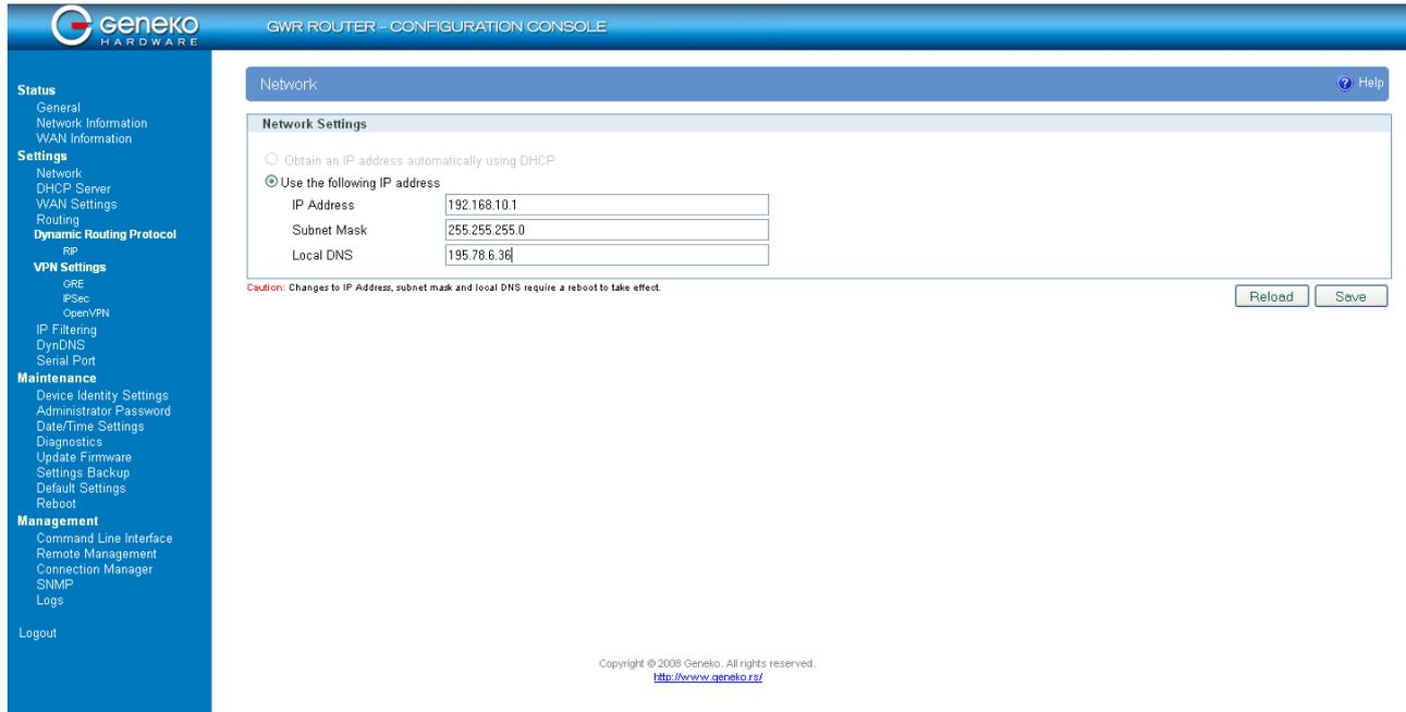
Figure 66 - Network configuration page for GWR Router 2
