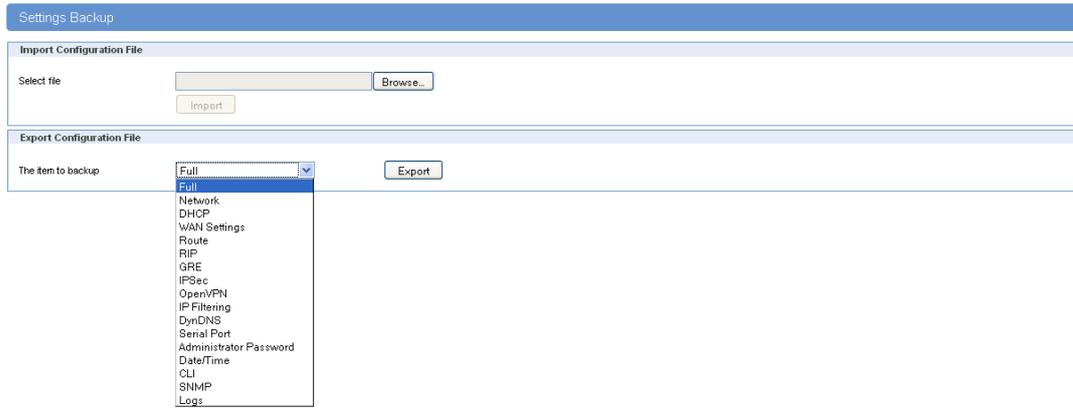
Figure 35 – Export/Import the configuration on the router
