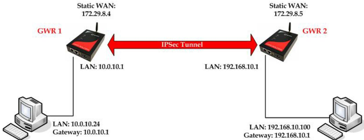
Figure 60 - IPSec tunnel between two GWR Routers
