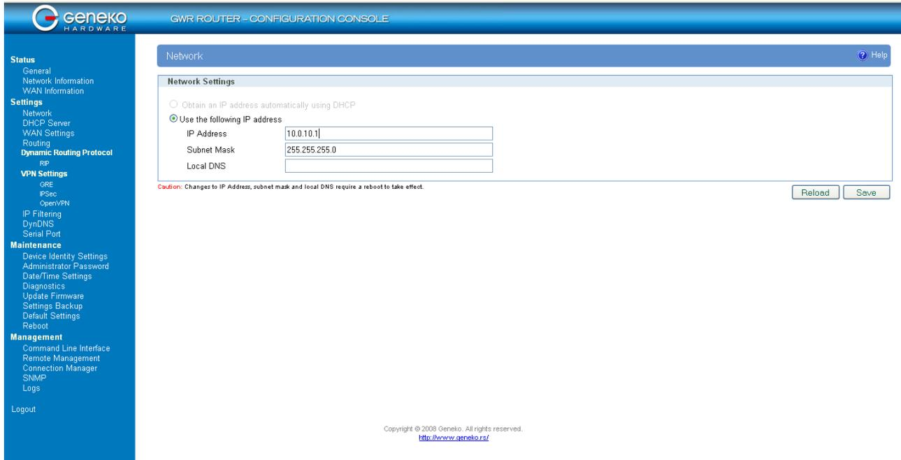
Figure 61 - Network configuration page for GWR Router 1
