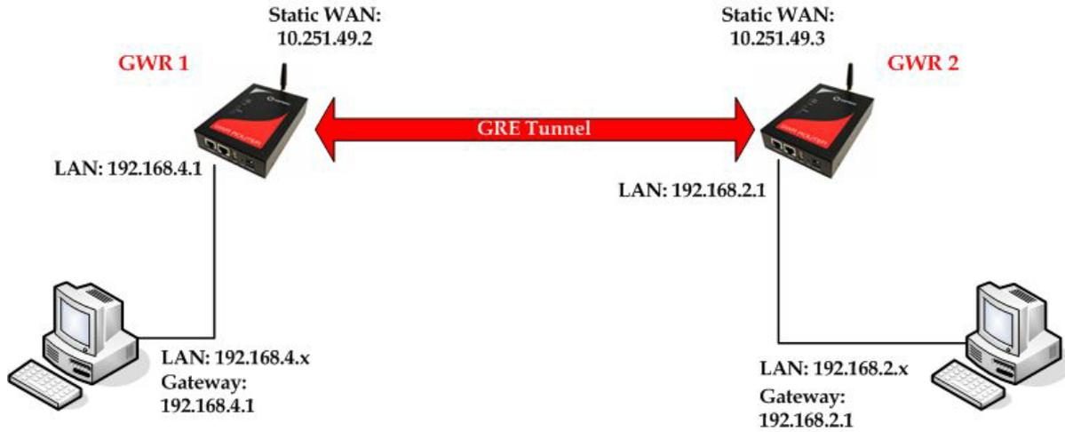
Figure 49 - GRE tunnel between two GWR Routers
