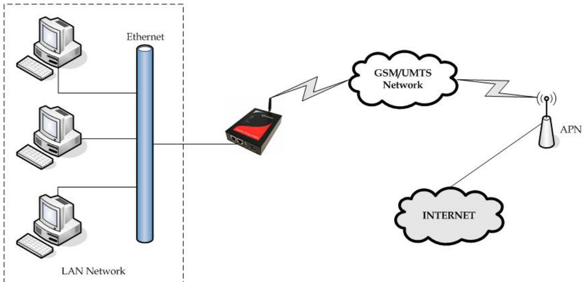
Figure 48 - GWR Router as Internet router
