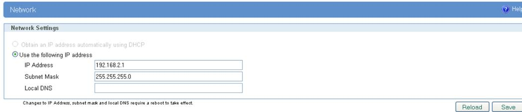
Figure 53 - Network configuration page for GWR Router 2
