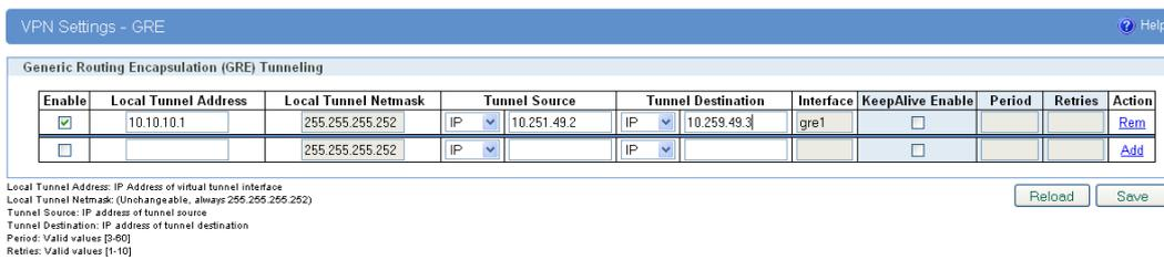
Figure 51 - GRE configuration page for GWR Router 1
