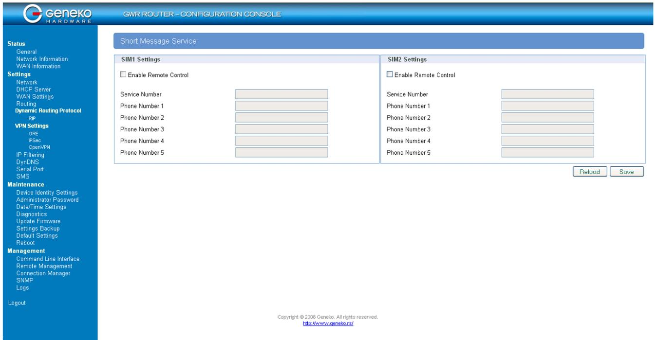
Figure 29- SMS remote control configuration
