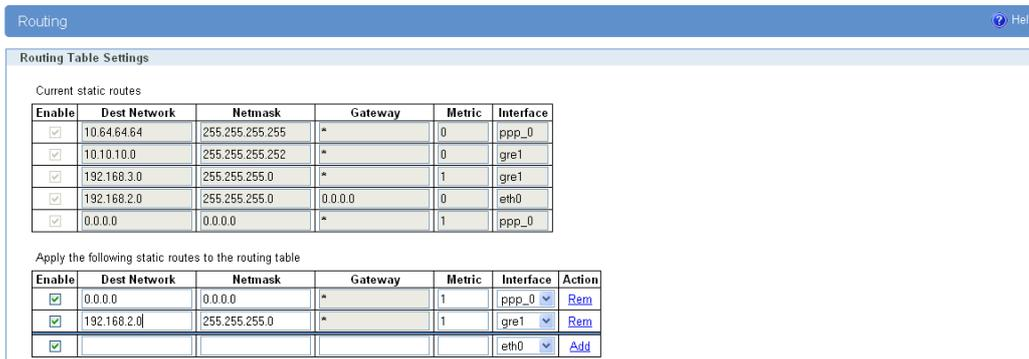
Figure 52 - Routing configuration page for GWR Router 1
