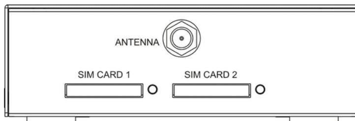
Figure 3 - GWR Router back panel (GPRS and EDGE)
