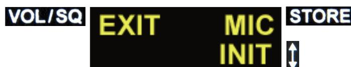
Therefore the INIT Menu is left with **VOL/SQ**. The device remains powered-on and returns to normal operation.
