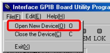
3. The **Open New Device** dialog box will appear. Then select the board model you want to use, the GPIB addresses, and termination method of the connected GPIB devices. Then click **OK**.
