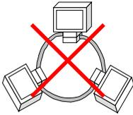
For reliable operations of a GPIB, you should not connect two cable assemblies without connecting a proper load or a GPIB device.
