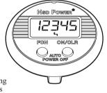
Press the "FCN" button to cycle through the display until the above symbol appears. Press the "ON/CLR" button once to clear the top speed for current session (⑤), press the "ON/CLR" button again to reset the historical top speed counter.
