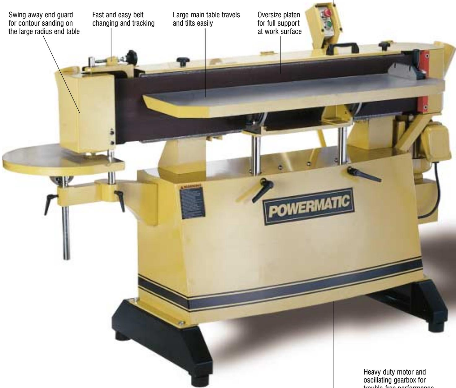
Swing away end guard for contour sanding on the large radius end table
