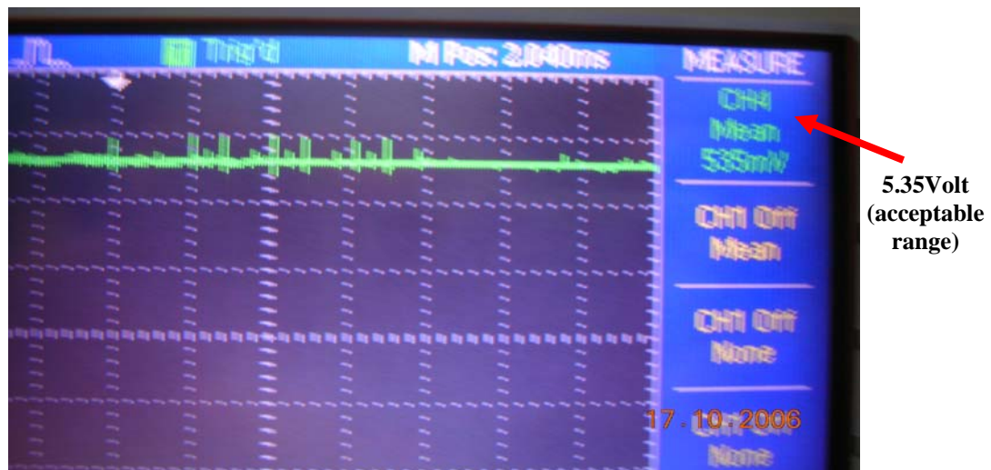
Figure 4.4 Measured Supply voltage for input processor board
