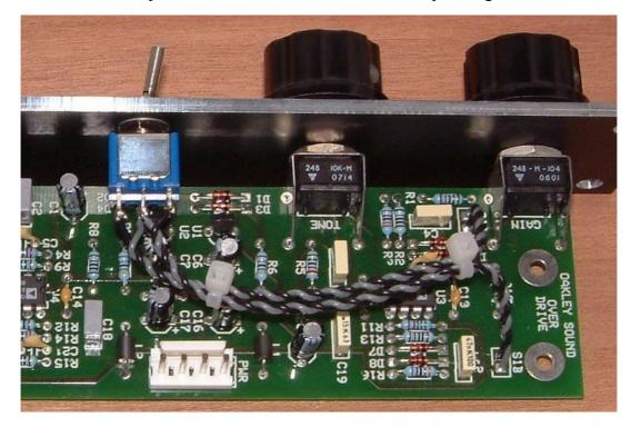
You can now use a couple of cable ties to hold the two twisted pairs together for neatness.
