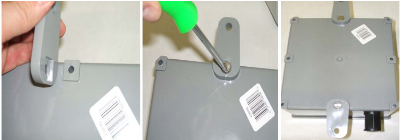
Figure 13: Attach Mounting Feet to the Remote Transmitter Module
