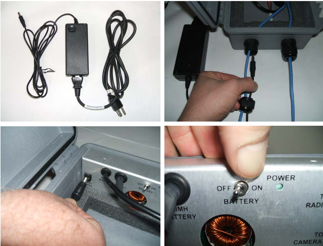
Figure 8: Using 36VDC Power Supply with Local AC Power
