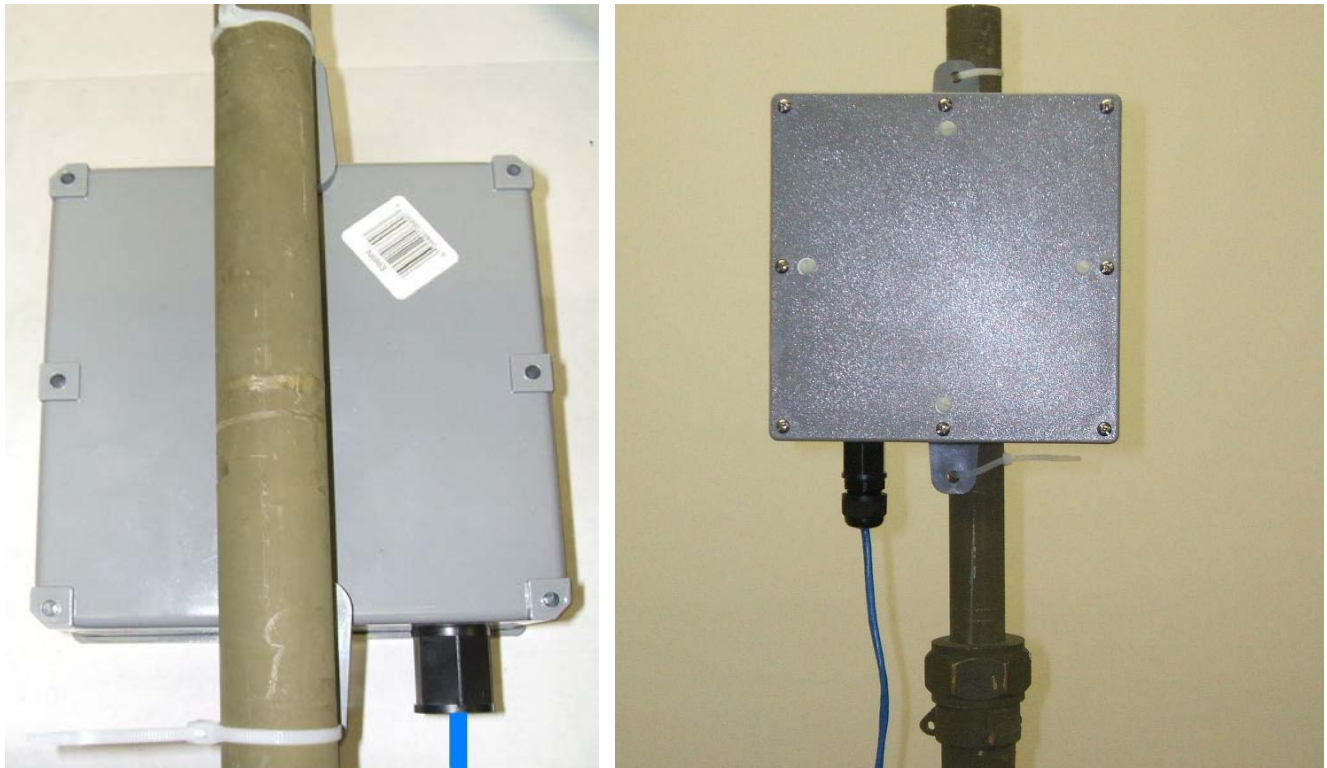
Figure 16: Pole Mounted Remote Transmitter Module
