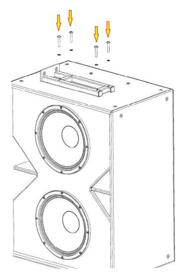
9. Repeat steps 5 to 7, securing the bracket to the left S215 subwoofer.
