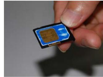
3. Unplug the pop-up slot, insert the SIM/UIM card, and please note the card missing angle should fit the slot.
