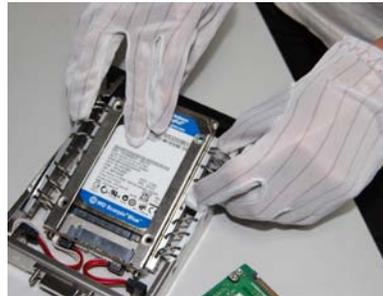
5. Please wear antistatic gloves. Carefully put in the first HD on the bracket (PCB face down), aim at the HD interface and insert it tightly.
