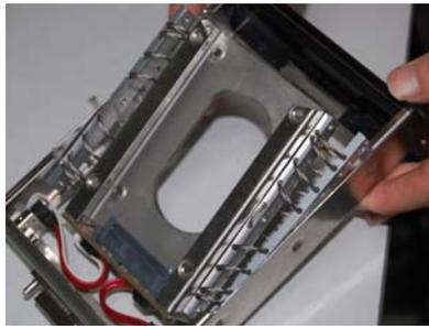
4. Upward Push out the HD bracket on the side of baffle with appropriate force.
