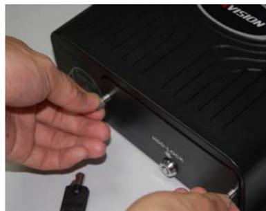
2. Firstly, open the HD-Lock with the key, and loosen the screw alone the anti-clockwise. Then pull out the HD box with uniform force.
