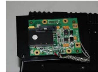
4. Insert the SIM/UIM card back to the module, and fasten the screws on the board.
