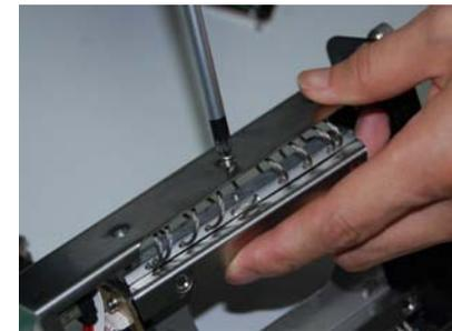
3. Remove the 6 screws used for fixing the HD bracket on the right and left sides.
