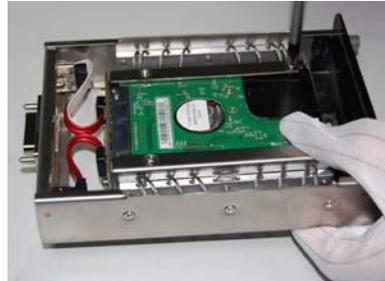
8. Install the HD screws, and fasten the HDs (4 screws per HD)
