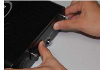
9. After the HD installation, push in the HD box and screw up. Don't forget to lock the HD-Lock.
