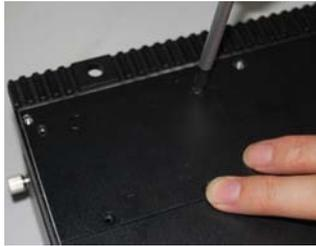
1. Reverse the device, loosen the screws of the wireless network module board on the right corner
