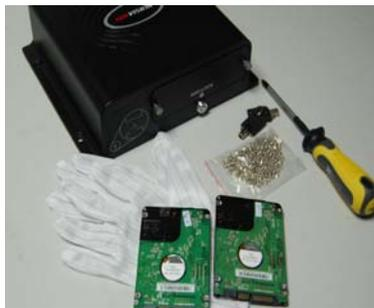
1. Please prepare all the tools and materials: 2.5 inch SATA HD, anti-static gloves, HDD-Lock key, cross screwdriver, HD screws
