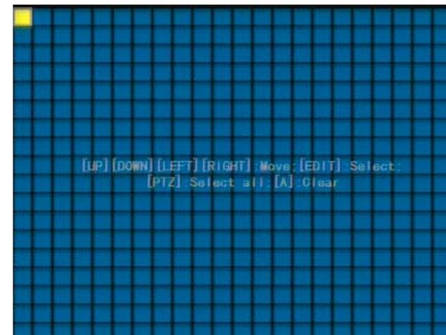
Fig.5.15 Motion Detection Area Setup
