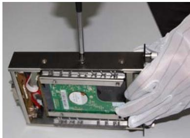
7. Restore the HD bracket position, aim at the holes and tighten the screws.
