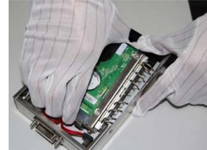
6. Put in the second HD on the bracket (PCB face down), aim at the HD interface and insert it tightly.
