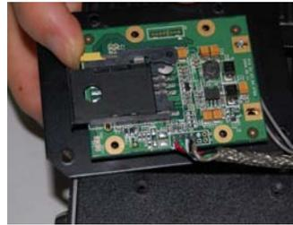
2. Carefully overturn the board with wireless module, use your finger press the yellow handspike softly (as shown). The slot will pop-up.
