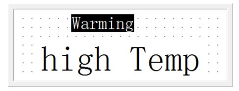
When the temperature, voltage, wind speed is too high, man-machine interface will report warnings to remind the owners.
