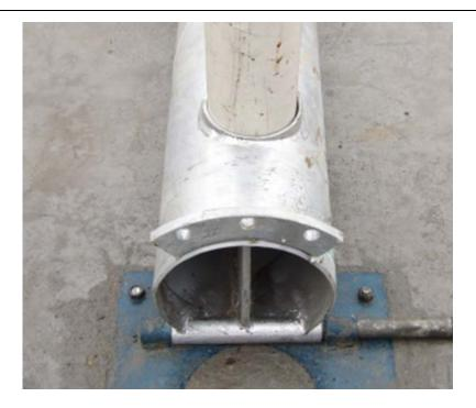
1. Connect each section of the pole by screw as below.
