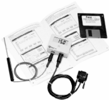
Figure 2: Connecting a sensor to an EasyLog module
